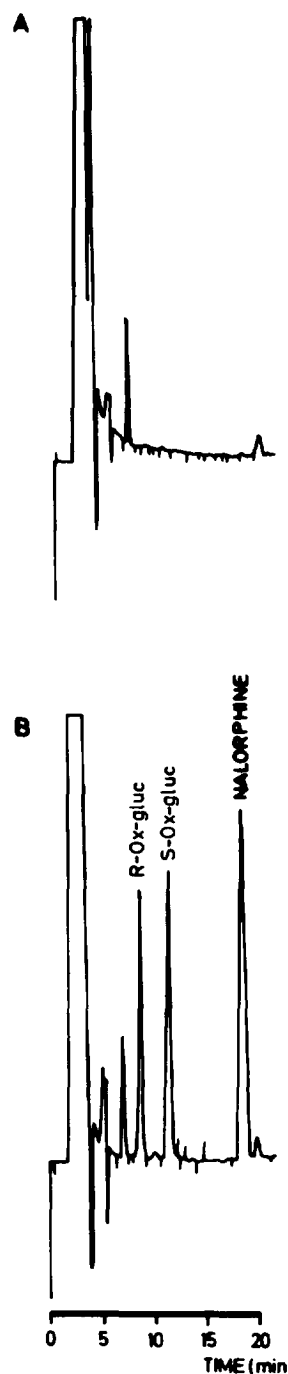
Fig. 1. Representative chromatograms obtained after incubation of rabbit liver microsomes with RS -oxprenolol. The microsomal suspensions are incubated with RS -oxprenolol for 40 min in the absence (A), and in the presence (B) of UDPGA.
